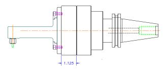
**Size IM Milling Style Angle Head:** A head suitable for milling (previously available for for Size 2 and 3 heads only) is now available for the Size I head also. The Size IM incorporates two preloaded bearings on the front of the spindle for improved performance and durability in side load applications. To order, simply add the "M" designation after the size designation in the part number (i.e. CV-40-1-**M-**2-1-1)
