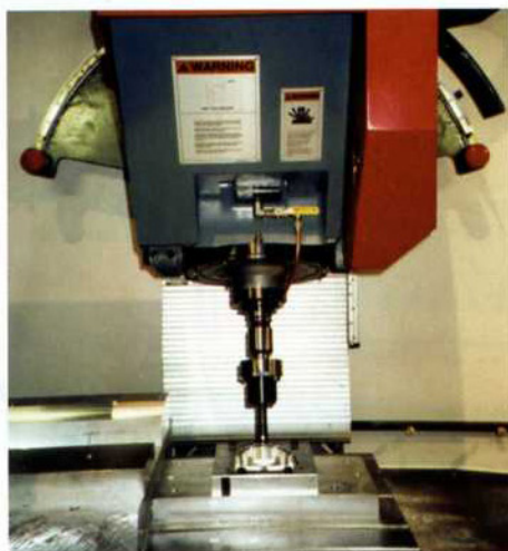
Left: Coolant-driven angle head drilling multiple rivet holes in a prototype leading wing frame component on a Cincinnati Machine V5 vertical machining center.
