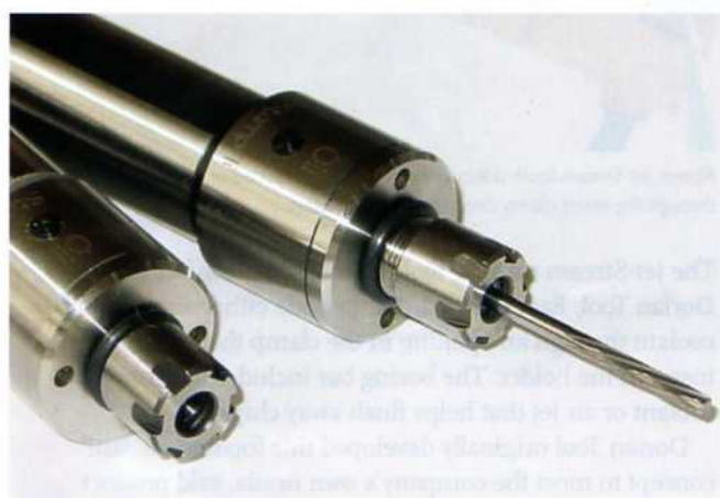
Above: Orbitally floating micro reamer chucks from Genevieve Swiss Industries.
