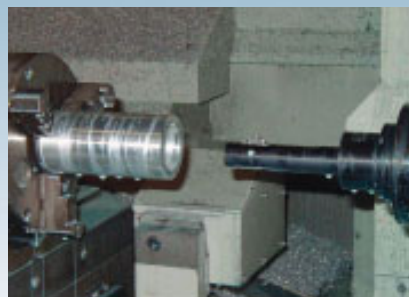
Cutting multiple keyways on a machining center.
