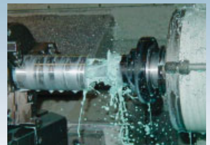
Cutting multiple keyways on a machining center.
